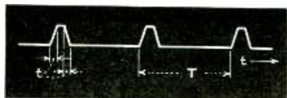
Fig. 5—Wave form of pulse requiring wide band amplifier for its transmission
