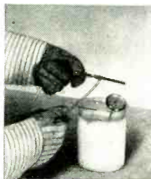
TRANSFLEX does not shatter when wrapped around a mandrel after removal from -50^{\circ}\text{C} . solution of dry ice and alcohol.
