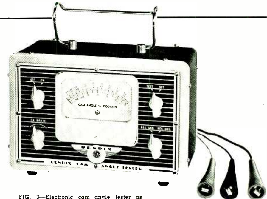
FIG. 3—Electronic cam angle tester as supplied to garage maintenance men
