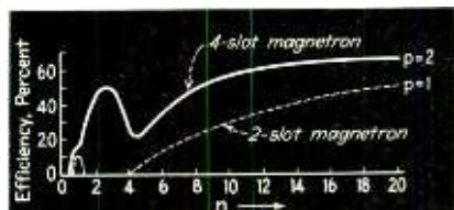
Fig. 13—Dependence of efficiency on the order of oscillation, n , for two magnetrons
